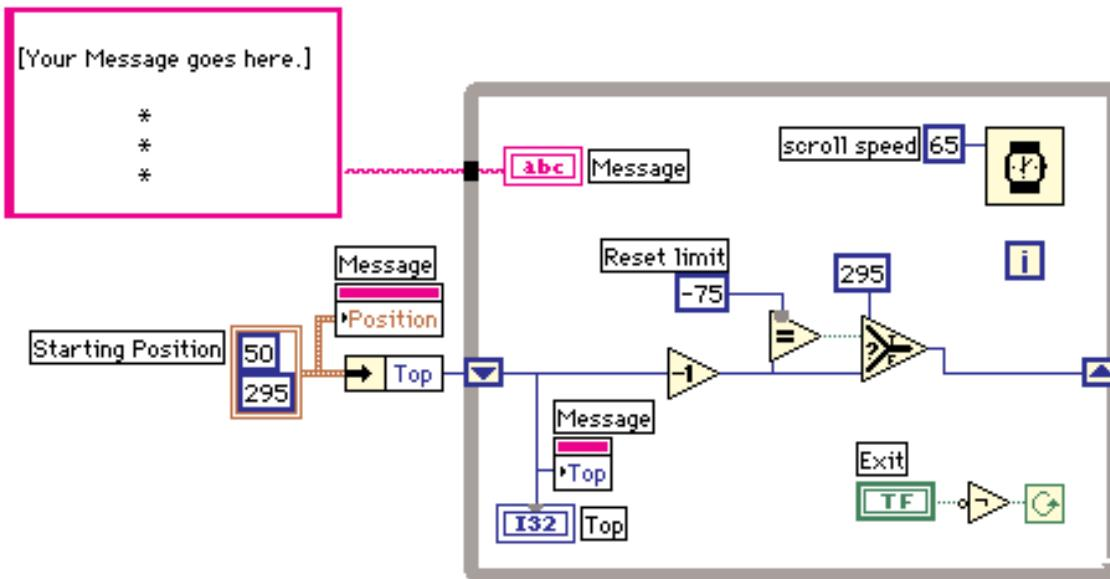
**Figure 3: Repeatedly decrementing the “top” parameter of the message “position” attribute node scrolls the text up the screen one pixel at a time. When the reset limit is reached, “top” is restored to the initial value of 295 and the process repeats.**
