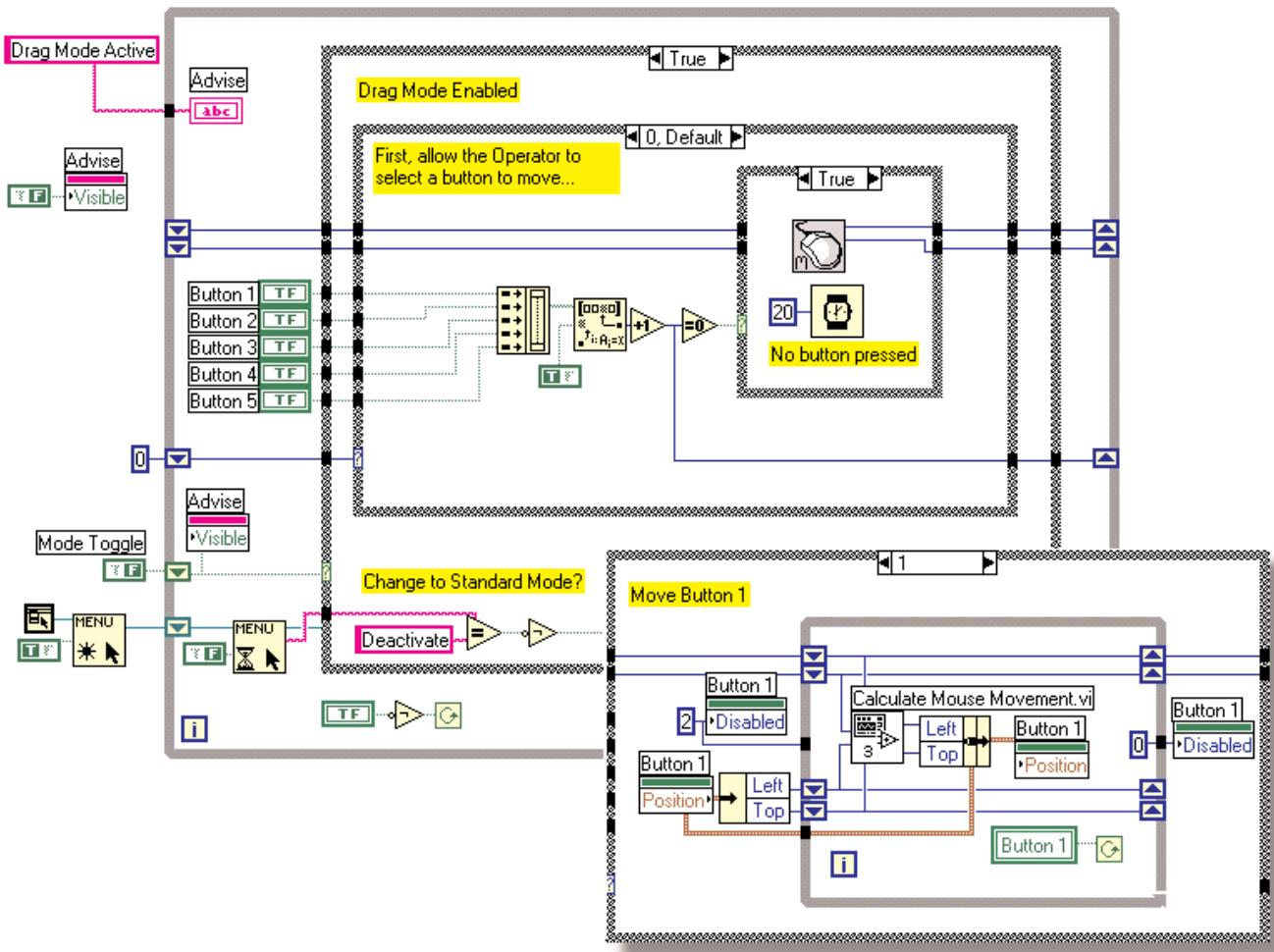
**Figure 2e:** After “drag mode” is activated from the Drag & Drop menu, the VI waits for one of the five buttons to be pressed (see 0, Default case above). When one of the five buttons is pressed, we proceed to the corresponding “button move” logic. The logic for button #1 is shown in the “case 1” inset.
