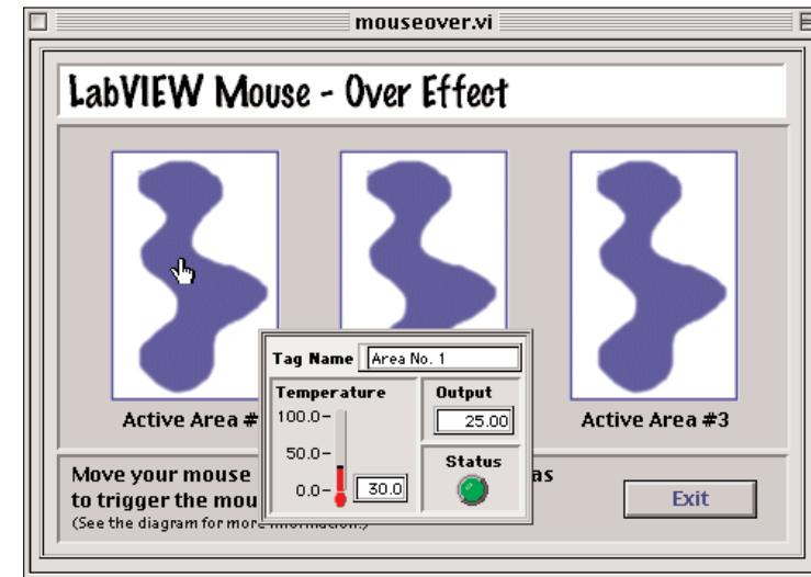
**Figure 1a:** As the mouse passes over one of three predefined "hot spots", a corresponding display cluster pops up to reveal hidden parameter values.
