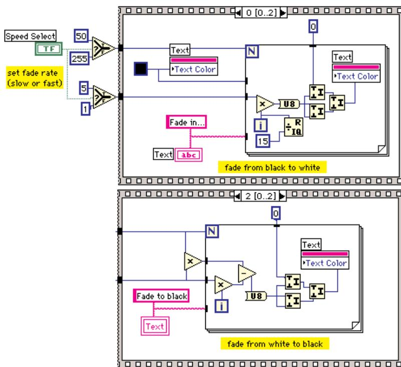
**Figure 4:** In frame 0 of the sequence structure (upper frame) you can see the logic required to fade text from black to white. After a short time delay in frame 1 (not shown), the sequence proceeds to frame 2 (lower frame) and the text fades back to black. In both cases, RGB “grayscale” values are created by loading R, G, and B values with the same number.
