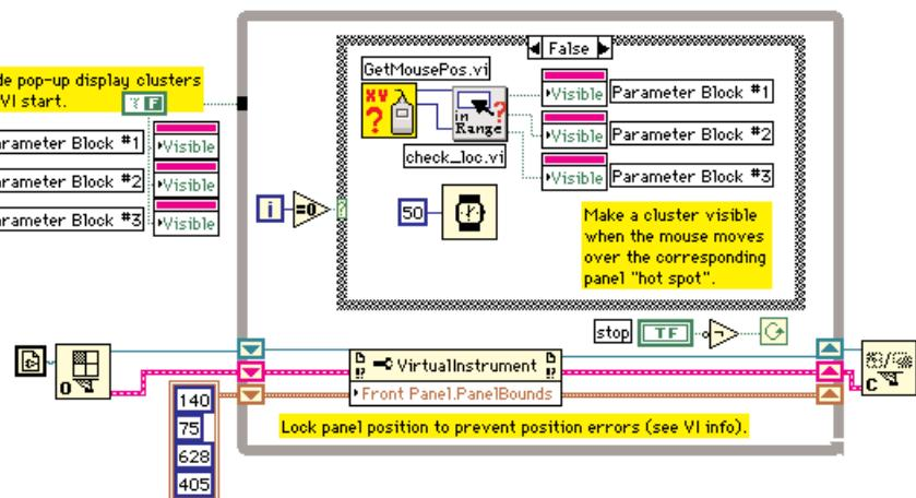
**Figure 1b:** The current mouse location is compared with the coordinates of predefined hot-spots inside check\_loc.vi. If a mouse-over state is detected, the corresponding cluster is revealed by setting its "visible" attribute to TRUE. Also notice that VI Server is used to prevent panel relocation at runtime.
