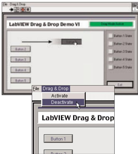
**Figure 2b:** Enter “drag mode” by clicking on “Activate” in the Drag & Drop menu.
